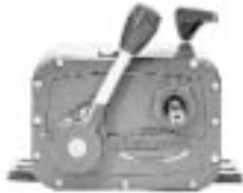
E Model 3 Torque Rating 12 in. lbs. Speed Range 400-0-400. Normal Input 1/4 - 1/3 H.P.
