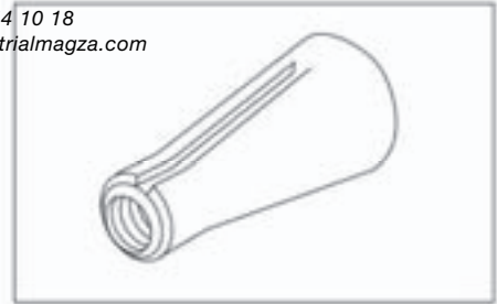
Tapered bore (4:1) - shaft tapers three inches per foot, for end of shaft mounting.
