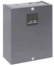
The TCS-168 power supply is designed to provide the correct power input to the TCS-310 Dancer Splicer Control and the TCS-320 Analog Splicer Control. Its switch selectable input allows the user to adapt to 120 or 240 VAC. It has dual voltage circuits to provide low voltage power and anti-residual output as well as power to operate two brakes. The TCS-168 is available with an enclosure or open frame for control panel mounting.
