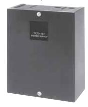
The TCS-167 power supply is designed to provide the correct power input to MCS-207, TCS-210, and TCS-220 tension controls. Its switch selectable input allows the user to adapt to 120 or 240 VAC. It has dual voltage circuits to provide low voltage power and anti-residual output as well as power to operate a brake. The TCS-167 is available with an enclosure or open frame for control panel mounting.
