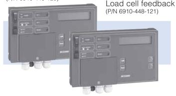
Both units have especially been designed for user applications. They include all functions for web tension control. The units are equipped with standard power supply, controller front face keyboard and display. The CTLC unit is provided with 2 load cell inputs with selectable sensitivity from 10 mV to 10 V, compatible with most sensors on the market.
