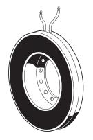
Since LK has a lower coefficient of friction, lower torque capability results. With LK facing, static torque capacity is only about 60% of catalog rating for any given size. So if a specific size clutch or brake is chosen for its rated torque capacity and LK facings are substituted for standard, a larger size unit will be needed to provide the same torque.
