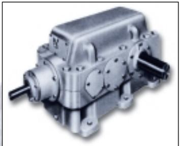
or vertical shaft up and down. This provides flexibility in space utilization for typical applications such as material handling or cooling tower drives. These units retain the Type TDS design features, including tapered roller bearings and heavy duty cast iron or welded steel housings. Nuttall Gear can supply drives separately or as a packaged assembly with motor and reducer mounted on a bedplate.
