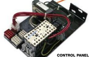
Provides easy access to controls, plug & play connectors allow for quick voltage change for dual voltage motors. Fuses located on terminal strip (optional).
