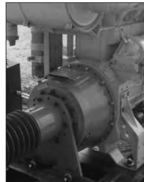
Wichita PTO mounted on Caterpillar diesel engine.
