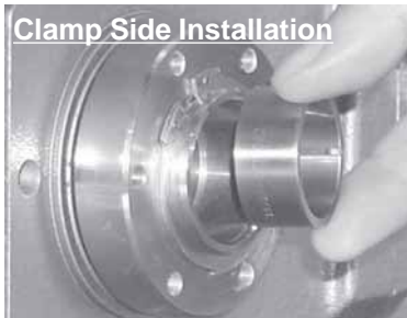
Insert Tapered Cone
