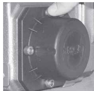
Install Closed Cover with the weep hole located at the lowest point.
