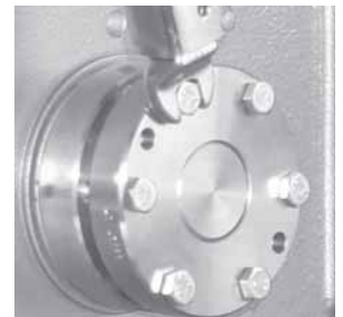
Use a Torque Wrench – see Table 1 for Tightening Torque
