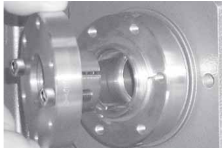
Install the Flanged Cone Assembly with it's slot opposite the slot in the tapered cone.
