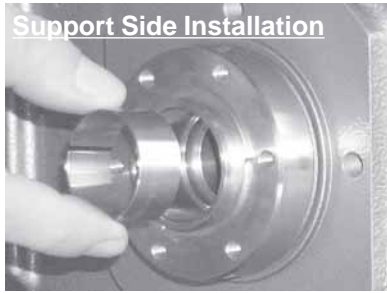
Insert Tapered Cone
