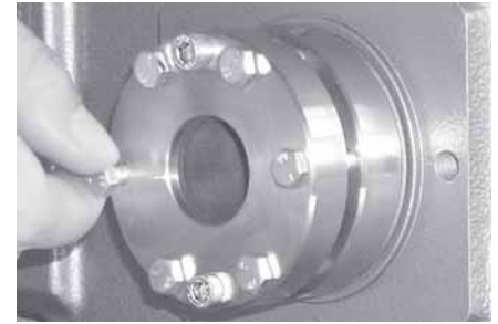
Hand Tighten Capscrews
