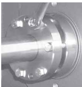
Tighten Capscrews – More Than 1 Rotating Sequence
