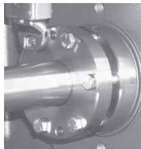
Use a Torque Wrench (See Table 1) for Tightening Torque
