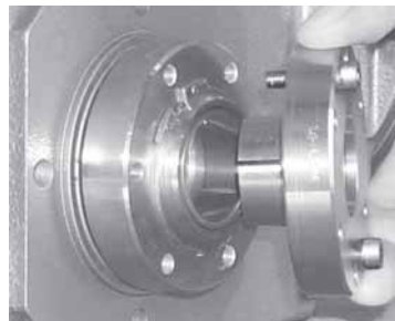
Install the Flanged Cone Assembly with it's slot opposite the slot in the tapered cone.
