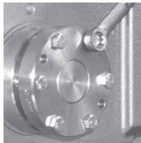
Tighten Clamp Side First – More Than 1 Rotating Sequence
