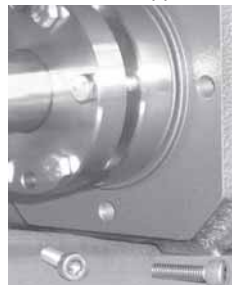
Remove the Spacer Bolts from both sides.
