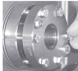
Hand Tighten Capscrews
