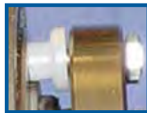
The spacer installed between the Support Side Bushing locking rings will not be removed but will compress as the capscrews are tightened.
