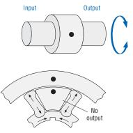
Any feedback torque from the **output member** is instantly stopped by the wedging of sprags between the fixed outer race and the **output member** feedback torque never reaches the **control member**. Special Purpose Clutches MEX (55) 53 63 23 31 MTY Res (Reverse-Locking) DIST. AUTORIZADO QRO (442) 1 95 72 60 ventas@industrialmagza.com
