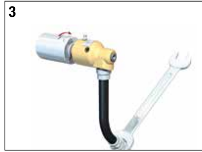
3 Connect flexible hose to supply line.
