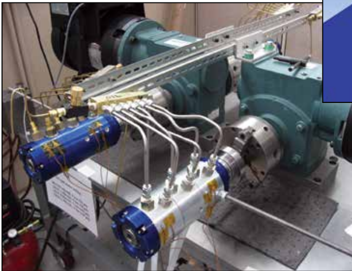
Deublin Multi-Passage unions testing fixture
