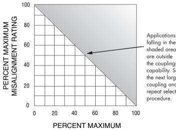
falling in the shaded area are outside the couplings capability. Select the next larger coupling and repeat selection procedure.
