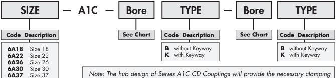
Note: The hub design of Series A1C CD Couplings will provide the necessary clamping force to hold the shaft in a dynamic application without the use of keyways.
