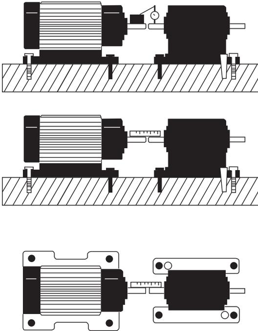
1. Use a straight-edge to check if the shafts are aligned with each other. For a more precise indication of alignment, use a dial indicator. (Figure 10)
