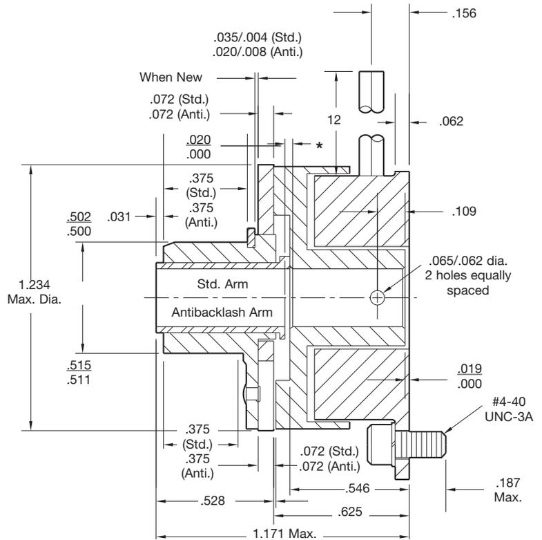
\* Mounting holes are within .006 of true position relative to pilot diameter.
