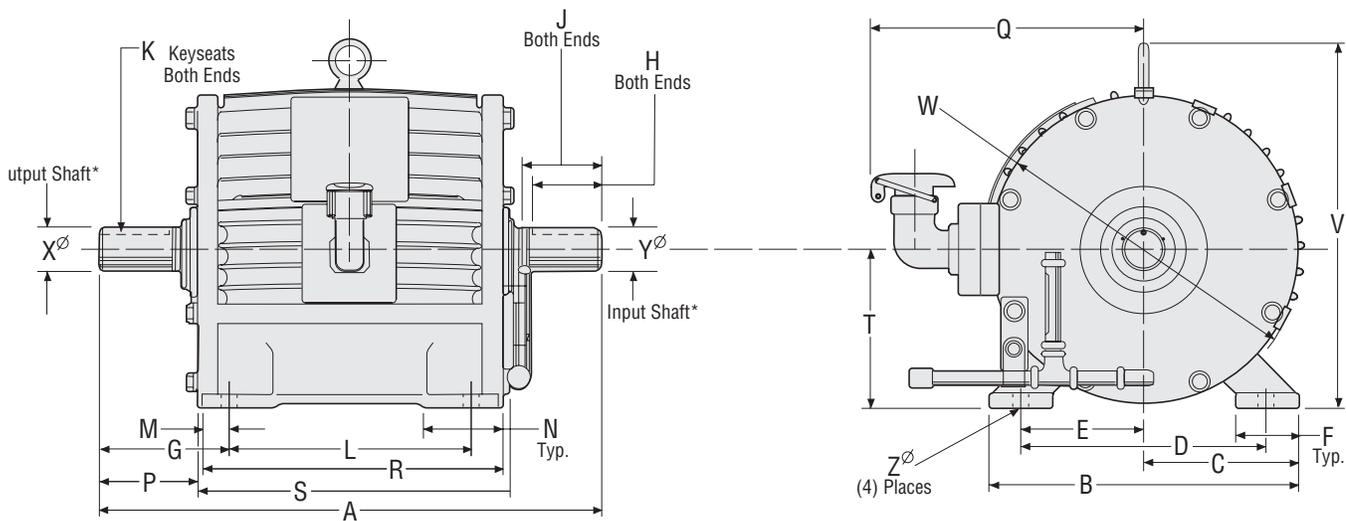
\*For C/T models, the input and output shaft diameters are reversed.
