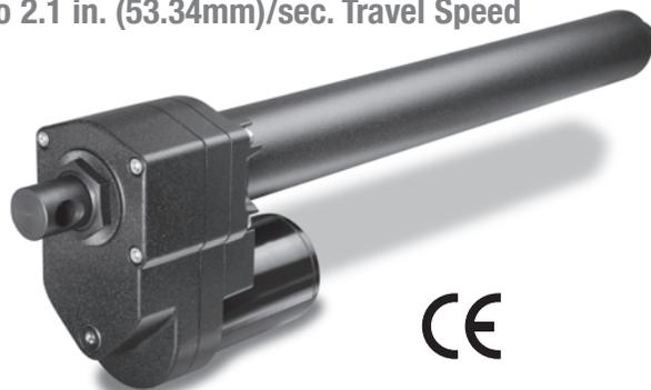
The K2x model provides the highest load rating in its class. This model incorporates all of the base K2 features with a ball nut screw for a 2,800 lb. (1270kg) load capability within a compact package size. The K2x includes a bi-directional wrap spring brake for load holding capability. These units are well suited for the most demanding applications where an alternative to hydraulic or air cylinders is needed or where hydraulic power sources are not available.
