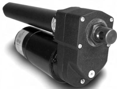
The K2x model provides the highest load rating in its class. This model incorporates all of the base K2 features with a ball nut screw for a 2,200 lb. (998kg) load capability within a compact package size. The K2x includes a bi-directional wrap spring brake for load holding capability. These units are well suited for the most demanding applications where an alternative to hydraulic or air cylinders is needed or where hydraulic power sources are not available.
