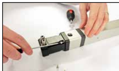
Tighten motor mounting screws
